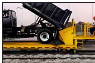
Ballast Spreading Hopper Spread ballast and level quickly with spreader bar
